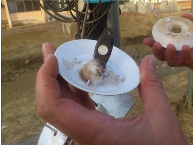
Figure 14: insects in and around moving parts, Ghana
